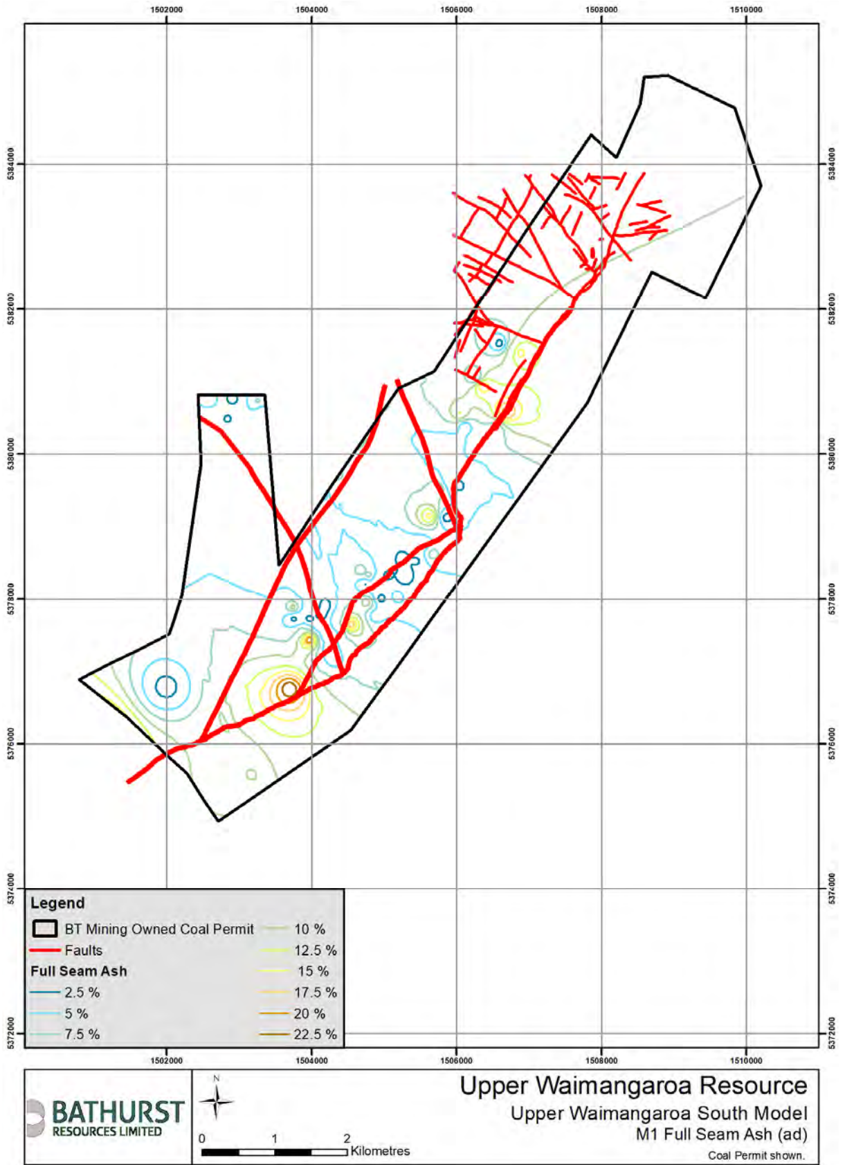
Figure 11: Plan showing in-situ full M1 seam ash on an air dried basis across the Upper Waimangaroa South resource
