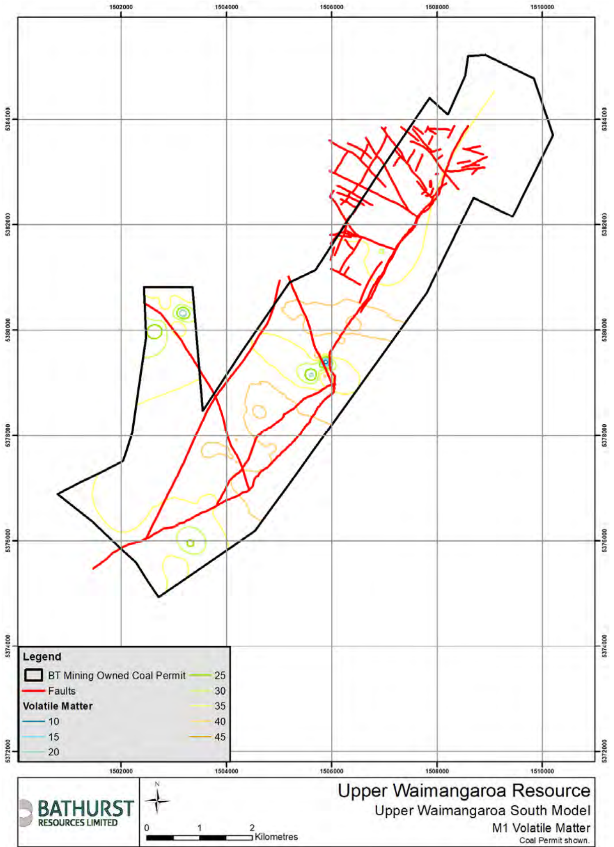
Figure 15: Plan showing full M1 seam Volatile Matter on an air dried basis across the Upper Wiamangaroa South resource
